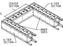
BRACKETS TO BE BOLTED TO UNDER SIDE OF CENTER UNIT WITH COAT ROD IN BETWEEN.
