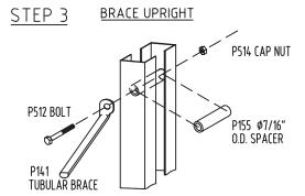
SET GATE ON FLOOR IN UPRIGHT POSITION AND EXTEND GATE TO ENABLE PLACEMENT OF \$\phi7/16 \text{ O.D. SPACER} BETWEEN PICKET CHANNELS. HOLDING THE SPACER IN PLACE, THREAD TUBULAR BRACE, PICKET CHANNELS, AND SPACER WITH Ø5/16 x 1-3/4" HEX HEAD CAP BOLT AND SECURE WITH Ø5/16" CAP NUT.
